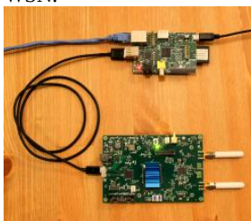
Figure 4. Interfacing of bladeRF and Raspberry Pi [6]
