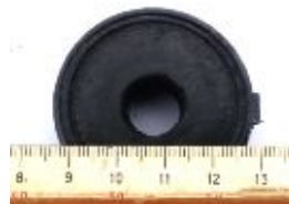
Fig. 2. The chopper wheel with hole with diameter of 15
